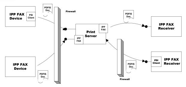
The IPP FAX device could communicate a PDF/IS encoded document to a PSI server outside of the firewall using either a PSI interface or an IPP interface. From there, the server could relay the document using the IPP FAX protocol; or the server could respond to a PSI poll by an IPP FAX receiver within a firewall.
