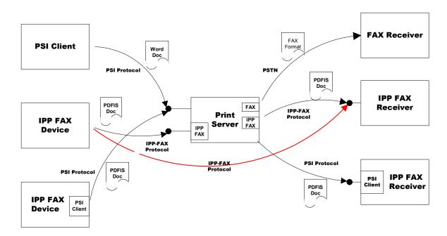
The coordination requires either that IPP fax needs to include a PSI interface or that the PSI Server needs to include IPP fax interfaces.
